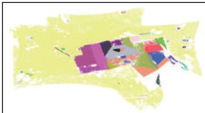
Figure 13. Segmented point cloud (extracted planar surfaces) over the area of interest
